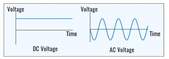
"DC" refers to "Direct Current" and means that the voltage is a constant. Typically, this is 12 volts DC on US fire apparatus. The DC electrical system relies on the Apparatus' Engine to be running to charge the batteries, which in turn supply power for the items attached to them. DC electrical systems are covered in NFPA 1901 & 1906 Standards, Chapter 13, "Low Voltage Electrical Systems"
