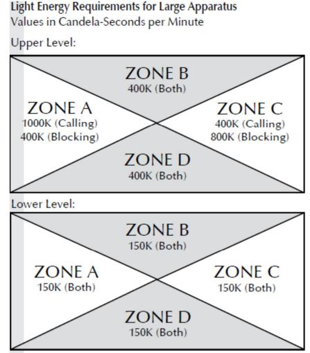
For vehicles 25 feet or longer the light output at each data point on the horizontal plane must be a minimum of 10K and 3.5K at  $\pm$ 5 degrees.
