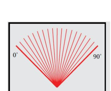
Each Zone on a Large or Small Apparatus consists of 19 data points (10,000 candela-sec./min.) where light energy is measured. See illustration above.
