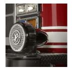
• Electronic Siren Speaker – This consists of an electro-acoustic transducer (speaker driver) which converts the electrical signal from the amplifier into acoustical energy. The speaker driver is enclosed within a housing to couple and amplify the projected acoustical output.
