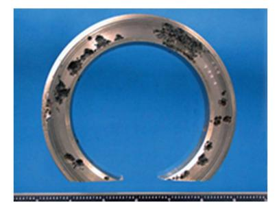
Pitting is a good example of Localized Corrosion often caused by uneven plating of the surface.
